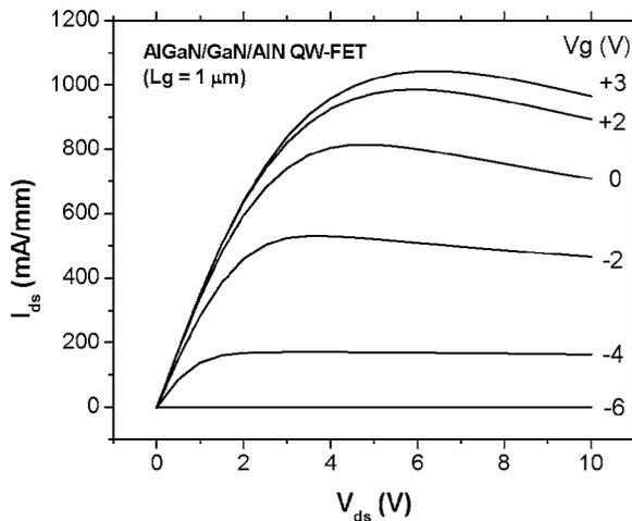
FIG. 3. dc characteristics of fabricated AlGaIn/GaN(50 nm)/AlN QW-FETs with 1  $\mu\text{m}$  gate length and 80  $\mu\text{m}$  gate width.
