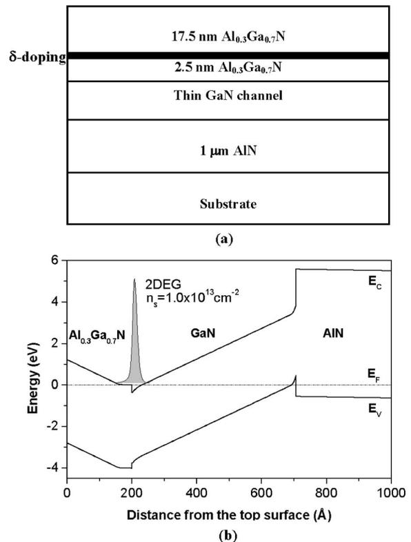
FIG. 1. The schematic diagram (a) and the simulated band diagram (b) of the AlGaN/GaN/AlN QW-FET structure used in this study. A Si  $\delta$ -doping level of  $4.5 \times 10^{12} \text{ cm}^{-2}$  and 50 nm GaN layer thickness are used for the calculation.
