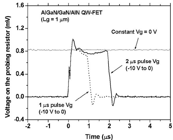
FIG. 4. Gate lag measurement performed for an AlGaIn/GaN(50 nm)/AlN QW-FET under pulse gate driving condition. The voltage on the probing resistor is proportional to the drain current. The drain current collapse is calculated by comparing the voltage under pulse driving with that of DC driving. In the measurement, the pulse has a frequency 100 kHz and pulse width 1  $\mu\text{s}$ .
